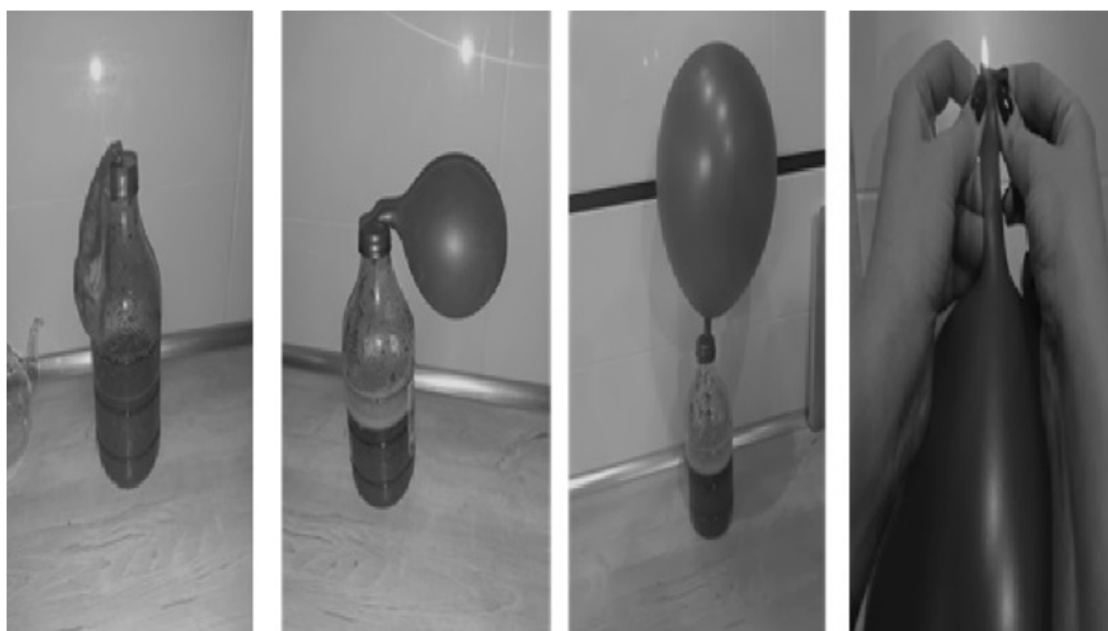
Fig. 1. – Collecting biogas and checking its availability using a match flame
